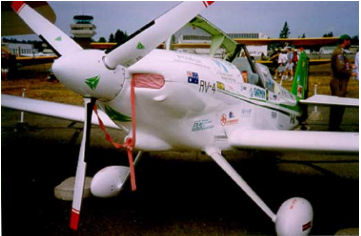
VH-NOJ from the front, showing the MT CS prop. Jon's in the background, talking to some interested spectators.
